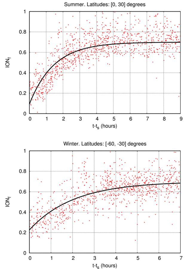
**Figure 9:** Two examples of best-fit curves (black solid lines) to  $ION_f$  values (red crosses). The horizontal axis is the time after sunrise at 350 km of altitude.
