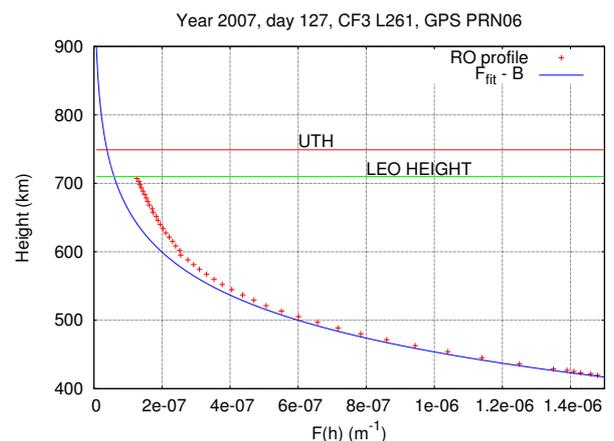
**Figure 2:** An example of the extrapolation strategy used to calculate  $EC_{\text{ion}}$ . Red crosses: a particular RO-retrieved shape function. Blue solid line: the extrapolated exponential term from equation (2) obtained after fitting the STIP model function. The red and green horizontal lines indicate, respectively, the UTH derived by the STIP model and the height of the CF3 satellite.
