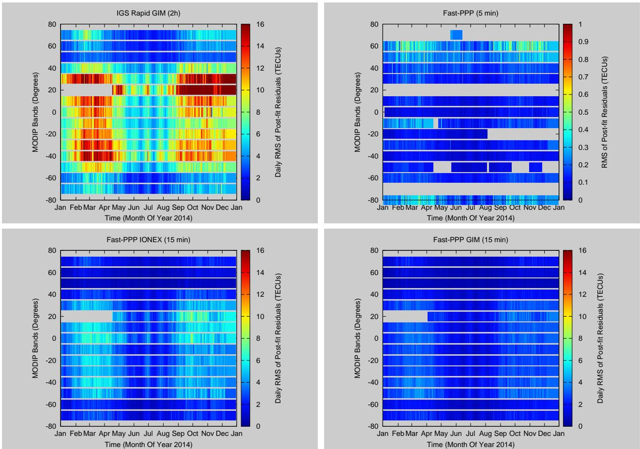
**Figure 3: Results of the consistency test between different GNSS ionospheric models along year 2014 for different MODIP latitudes. The upper left plot corresponds to the 2-h Rapid IGS GIM, the upper right plot to the real-time 5-min two-layer Fast-PPP model. In the bottom row, the 15 min Fast-PPP GIM are stored in IONEX format (left, geographical latitude interpolation) and using the MODIP interpolation (right). The color band in every plot indicates the range of the errors.**
