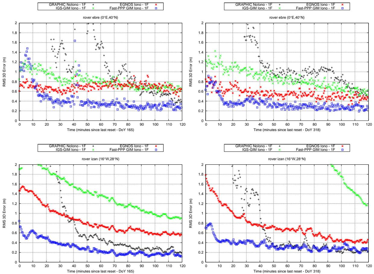
**Figure 4: Single-Frequency Navigation results: RMS of the 3-D error as a function of time since the user receiver is reset (with resets every 2 hours and 12 resets merged per day) for rover ebre (top) and izan (bottom) for DoY 165 (left) and 318 (right) of year 2014. In each plot, the ionosphere-free single-frequency solution GRAPHIC (black) is compared with the enhanced positioning using the ionospheric determinations from the Fast-PPP GIM (blue), IGS-GIMs (green) and EGNOS (red).**
