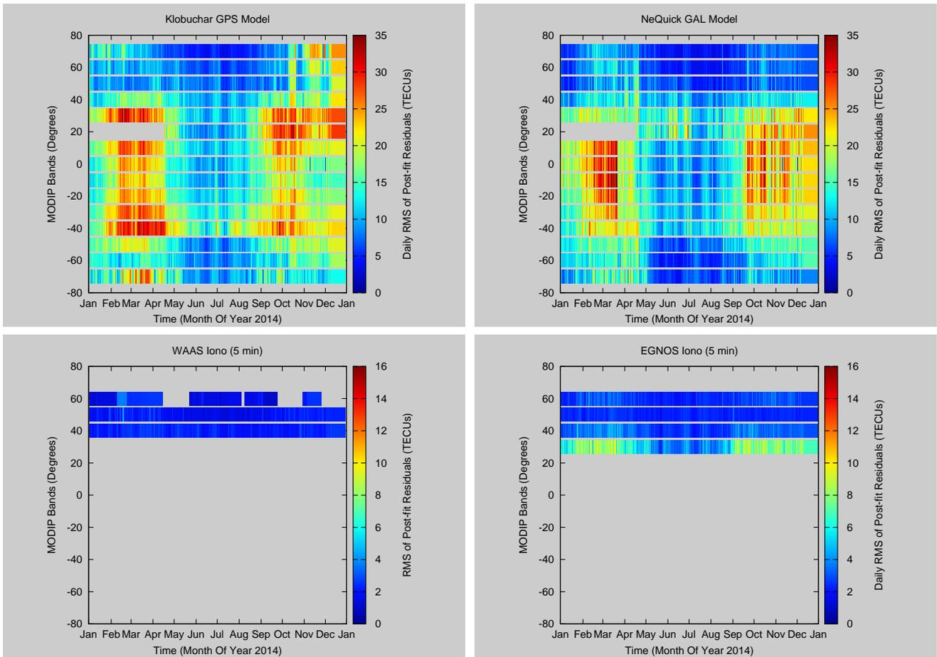
**Figure 2: Results of the consistency test between different operational GNSS ionospheric models along year 2014 for different MODIP latitudes. The top row shows the absolute value of the error of the GPS (left) and NeQuick Galileo (right) broadcast models, while the bottom row represents the real-time (5 min) ionospheric corrections of the augmentation systems WAAS (left) and EGNOS (right). The color band in every plot indicates the range of the errors.**
