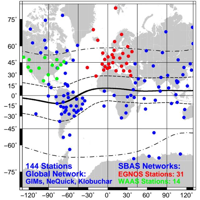
**Figure 1: Distribution of permanent receivers used to assess ionospheric models during 2014. All stations participate in the assessment of global models: GIMs, Klobuchar (GPS) and NeQuick (Galileo). The red and green sub-set of receivers are used to assess the real-time ionospheric corrections of EGNOS and WAAS, respectively. The black curves indicate different MODIP latitudes: 0° (solid), ±36° (dashed), ±60° (dash-dots).**
