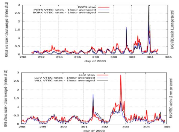
Figure 1: Comparison of the post-fit residuals RMS of an ionospheric model (red) and the RMS of AATR (blue and black) for two selected receivers. Left plot is for POTS sub-network (receivers POTS and BORK with 445km of baseline). Right plot is for LLIV sub-network (receivers LLIV and VILL with 544km of baseline).
