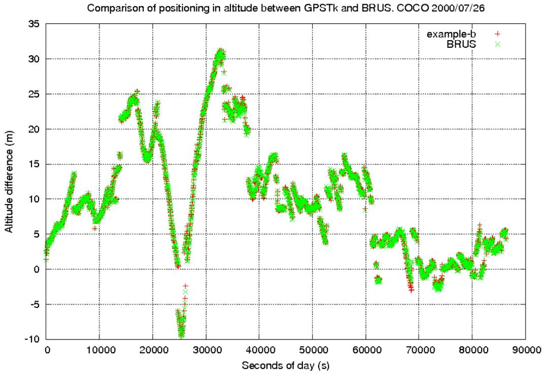
Figure 7: Comparison of vertical error between example-b and BRUS. COCO 2000/07/26.
