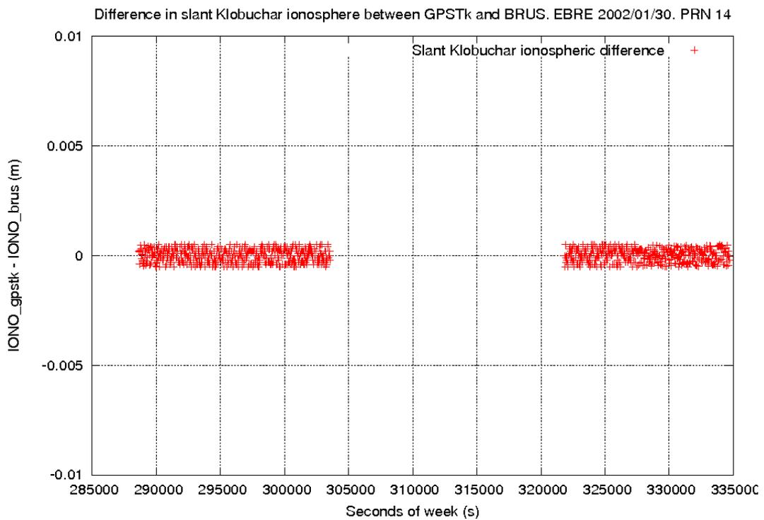
Figure 10: Difference in slant Klobuchar ionospheric modeling between example-b and BRUS. EBRE 2002/01/30. PRN #14.
