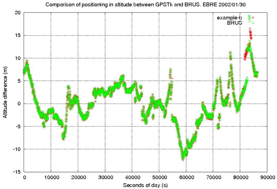
Figure 5: Comparison of vertical error between example-b and BRUS. EBRE 2002/01/30.
