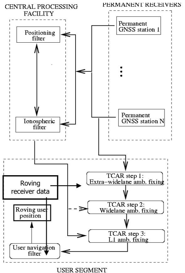
**Figure 1:** Layout of the original WARTK-3 algorithm, which incorporates the accurate real-time ionospheric corrections to the TCAR approach of solving the ambiguities from the longest to the shortest wavelength in a geometry-free way (see details of the WARTK-3 approach at Hernández-Pajares et al. 2003b).
