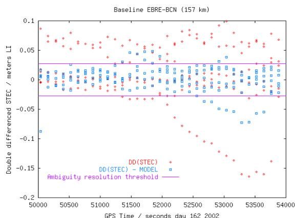
**Figure 5:** Double differenced STEC values (red) of the roving receiver, and the corresponding residuals after applying the reference net broadcast values (blue), for more than one hour in the UNBAR01 experiment.
