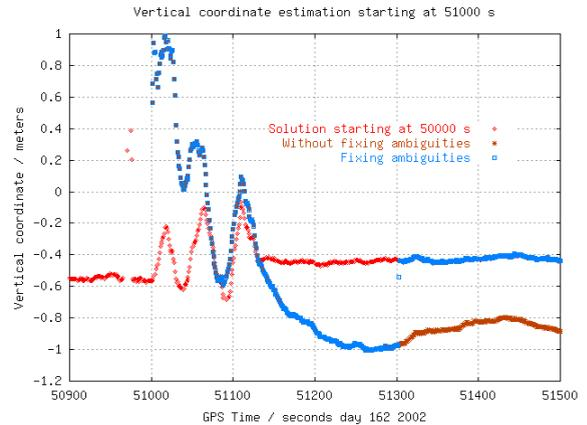
**Figure 8:** Plot similar to the last plot, showing the vertical component (Up), but after a general lost of satellites, fixing ambiguities at 51300s (blue) and floating ambiguities (brown).
