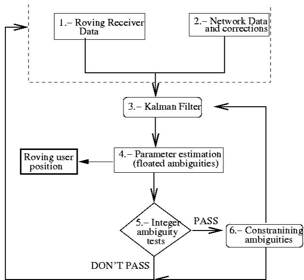
Figure 3: WARTK-3.2 algorithm layout for the roving user.
