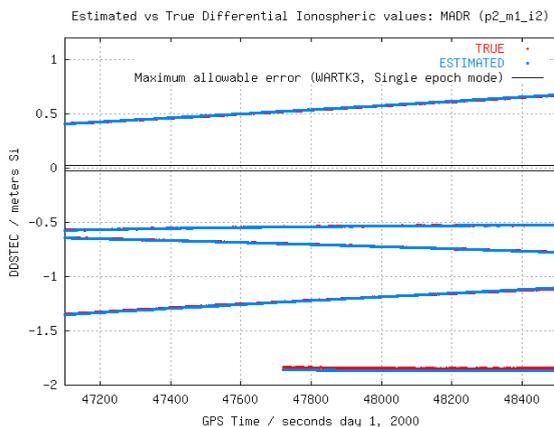
**Figure 24:** Estimated (blue) vs. actual differential ionospheric values corresponding to the satellites in view from the fixed station MADR treated as rover at more than 400 km from the nearest reference site (scenario (b)).
