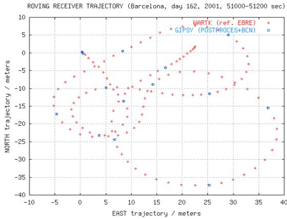
**Figure 6:** Roving car trajectory (North-East), corresponding to the same experiment, but with the car in movement, for two minutes. The red trajectory has been computed with WARTK being the closest station, Bellmunt, at 67 km away. And the reference trajectory (blue) is computed with GIPSY software (in post-process and using very close reference station data).
