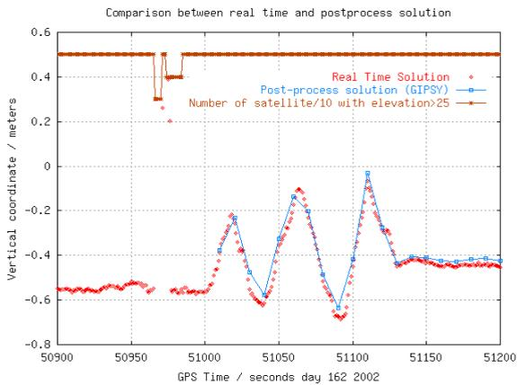
**Figure 7:** Plot showing the vertical component (Up), for five-minutes of the car movement in the UNBAR01 experiment. It corresponds, approximately, to the horizontal movement estimated in
