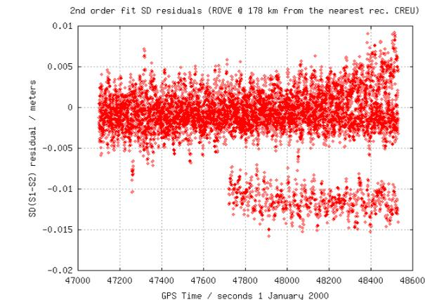
**Figure 13:** Double-differenced ionospheric refraction user errors when a second-order (quadratic) fit is used in the interpolation (scenario (a)).
