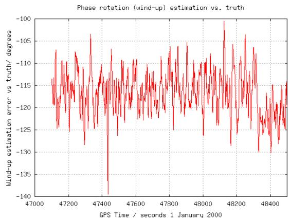
**Figure 19:** Errors (including an arbitrarily initial orientation value) of the antenna rotation instantaneous estimation for car ROVE in scenario (a).
