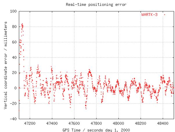
**Figure 25:** Vertical coordinate error of WARTK-3.2 for the fixed station MADR treated as rover at 404 km away from the nearest reference site (EBRE) and in Solar Maximum ionospheric conditions.
