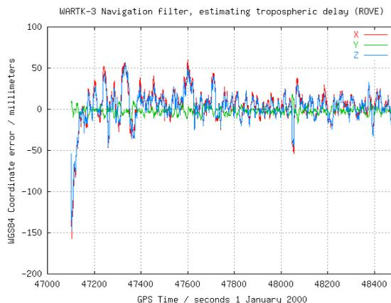
**Figure 14:** ROVE WARTK3 Navigation: X,Y,Z errors (scen. a).
