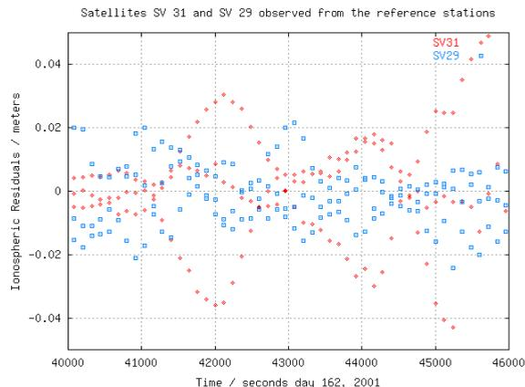
**Figure 4:** Ionospheric residual (true-planar fit model) computed at the reference stations for satellites SV/PRN31 (red crosses) and SV/PRN29 (blue squares).
