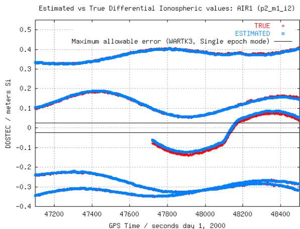
**Figure 20:** Estimated (blue) vs. actual differential ionospheric values corresponding to the satellites in view from the rover AIR1 (scenario (b)).
