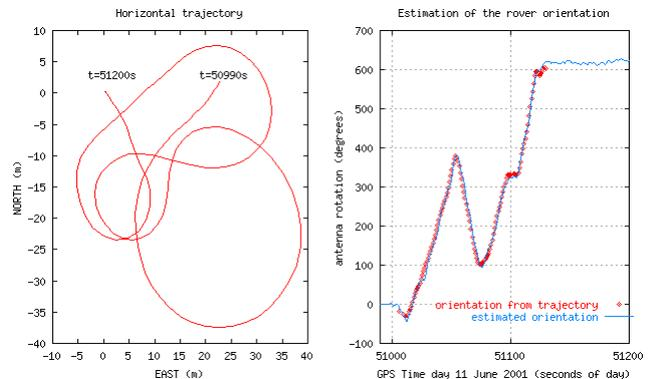
**Figure 9:** Plots showing the horizontal movement of the roving receiver, during a part of the UNBAR01 experiment (left side plot). At the right hand plot, the corresponding wind-up estimation (blue) compared with the value derived from the trajectory (red) are shown.
