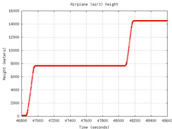
**Figure 23:** Height evolution corresponding to the GNSS receiver (AIR1) on-board an aircraft, in scenario (b).
