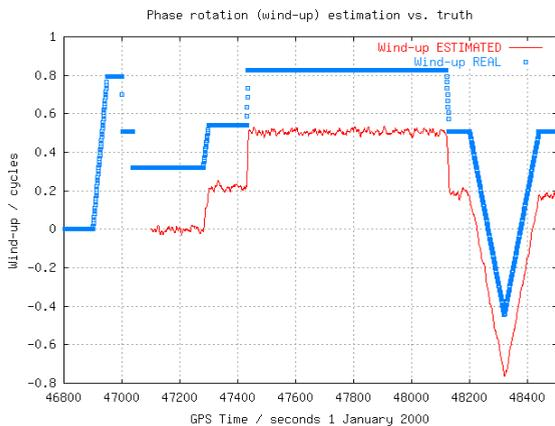
**Figure 17:** Real-time phase orientation change estimation (wind-up) in ROVE (red) vs. the real one (blue).
