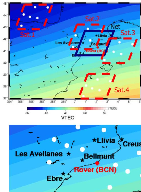
**Figure 2:** Regional network of the stations (dark stars) involved in the GPS experiment UNBAR01 (general view, topside, zoom, bottomside). Such stations have been used to test the new algorithms proposed in this paper. The roving stations were
