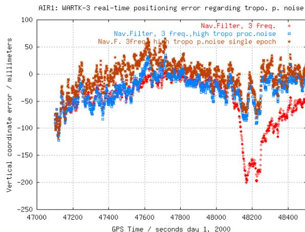
**Figure 22:** WARTK-3.2 Vertical coordinate error compared between using a standard ground-based tropospheric random-walk process noise (red), and using a higher process noise (blue and brown in single-epoch mode as well).
