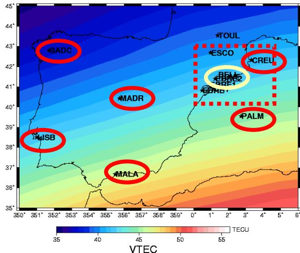
**Figure 10:** Scenario (a) layout –yellow ellipse=rover, red ellipse=fixed-.
