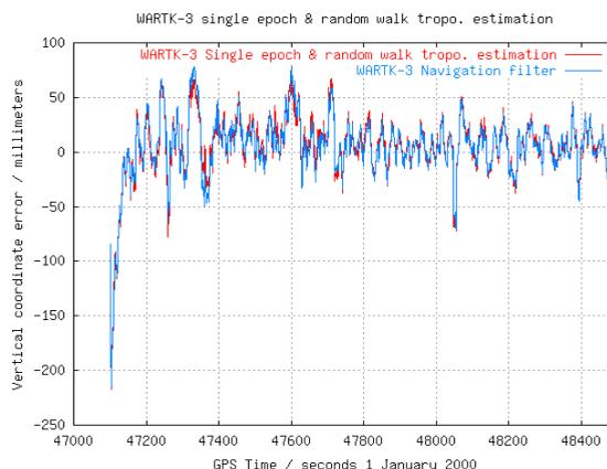
**Figure 15:** ROVE WARTK3.2 single-epoch Navigation treating the vertical tropospheric wet delay such as a random walk (X,Y,Z errors, scenario (a)).
