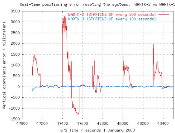
**Figure 16:** WARTK3.2 vs WARTK-2 WGS84 Vertical (up) positioning error for ROVE in scenario (a), starting up everything each 100/300 sec. respectively (including tropo.).
