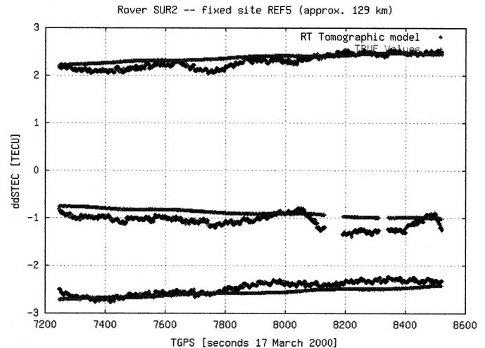
Fig. 1. Double-differenced STEC estimated in real time with the tomographic model, compared with the observed values for the surface roving receiver SUR2 referred to the most distant receiver, REF5 (about 129 km away from the rover).
