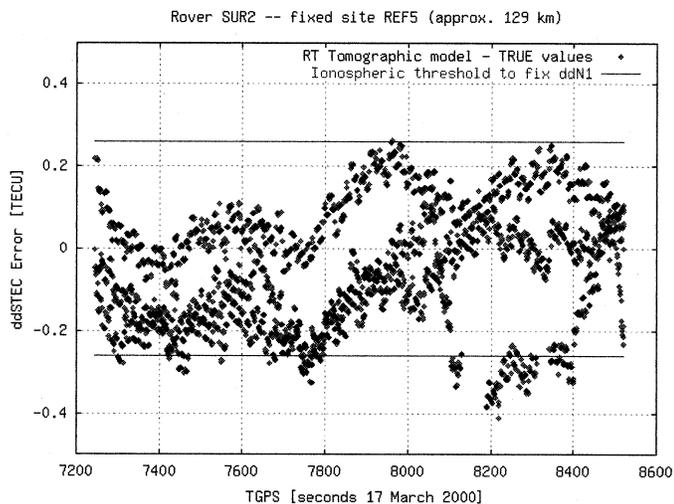
Fig. 2. Error in the real-time tomographic determination of the double-differenced STEC. More than 92% of errors fall between the critical  $\pm 0.26$  TECU levels (horizontal lines).
