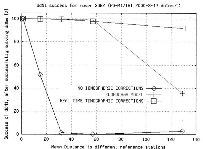
Fig. 3. Relative success of complete ambiguity resolution for the roving surface receiver SUR2, as a function of the distance to the reference station.
