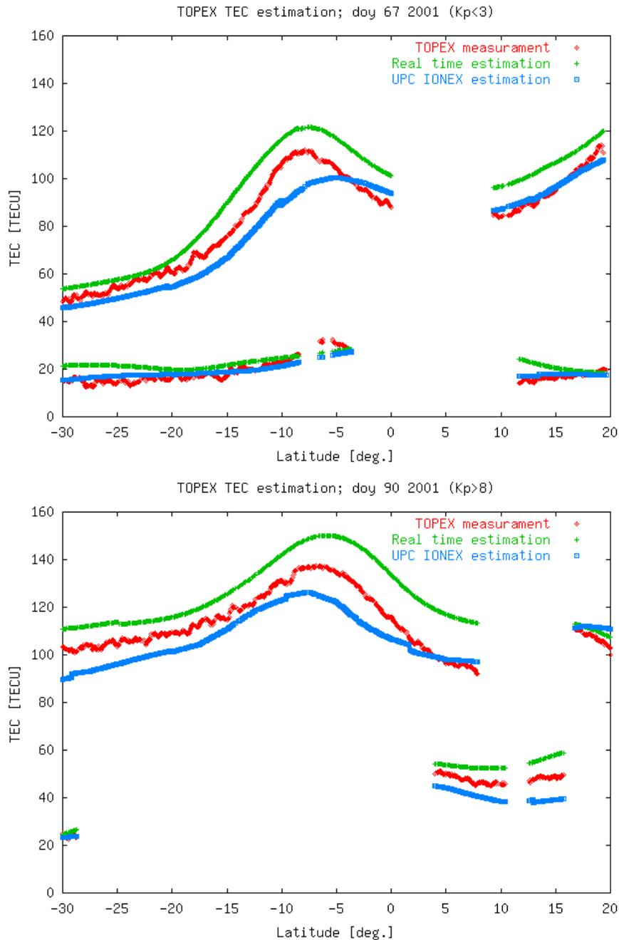
**Figure 5:** Comparison of real-time ionospheric vertical TEC determination, and post-processed solution, both with GPS data, and TOPEX TEC for a geomagnetically quiet day (March 3<sup>rd</sup>, 2001, top plot), and a day geomagnetically very disturbed, with  $K_p \cong 8$  (March 31<sup>st</sup>, 2001, lower plot).
