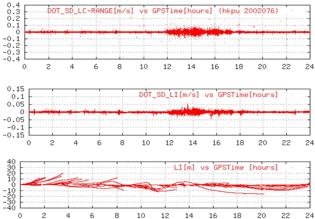
**Figure 10:** GPS receiver HKPU during day 076, 2002: Derivative of the prefit LC residual (single differences between satellites) at top; derivative of the corresponding ionospheric (geometric free) single differences (center) and plain ionospheric observations (bottom).
