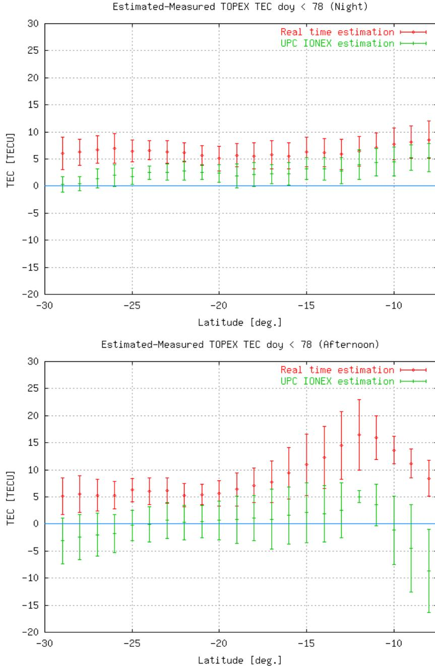
**Figure 6:** Bias and standard deviation (represented as bar errors) of the differences between GPS TEC and TOPEX TEC for the first part of the studied period with low geomagnetic activity (before DOY 78, March 19<sup>th</sup> 2001), during the local night (22-04LT) and during the local afternoon (12-18LT). Similar results are obtained with higher geomagnetic activity (starting on DOY 78).
