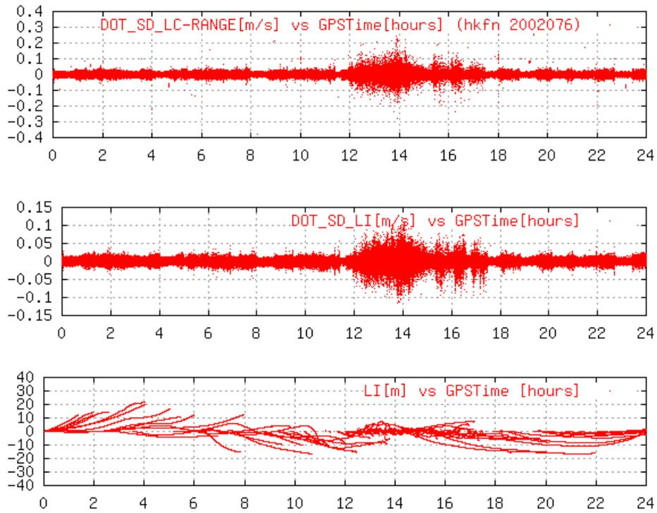
**Figure 9:** GPS receiver HKFN during day 076, 2002: Derivative of the prefit LC residual (single differences between satellites) at top; derivative of the corresponding ionospheric (geometric free) single differences (center) and plain ionospheric observations (bottom).
