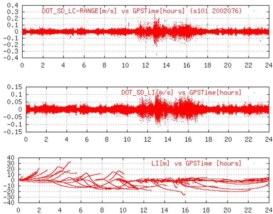
**Figure 11:** GPS receiver S101 during day 076, 2002: Derivative of the prefit LC residual (single differences between satellites) at top; derivative of the corresponding ionospheric (geometric free) single differences (center) and plain ionospheric observations (bottom).
