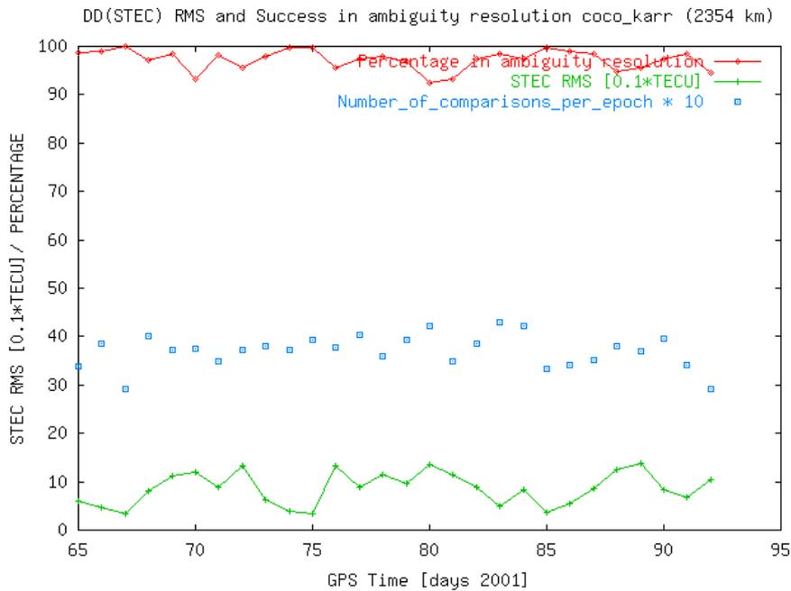
**Figure 8:** An example of the RMS of the  $\nabla\Delta STEC$  real-time determination, and associated success for the double differenced widelane ambiguity, for the baseline from COCO (in the southern Appleton anomaly footprint) to KARR in Australia (2354 km away, bottom plot) since 6 March to April 2, 2001. The mean number of observations is also plotted for each day.
