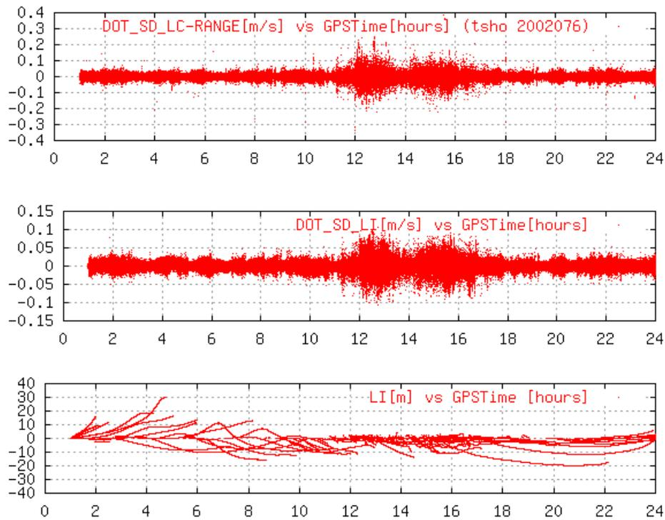
**Figure 12:** GPS receiver TSHO during day 076, 2002: Derivative of the prefit LC residual (single differences between satellites) at top; derivative of the corresponding ionospheric (geometric free) single differences (center) and plain ionospheric observations (bottom).
