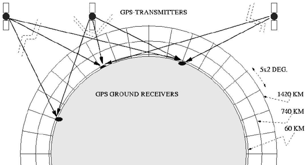
**Figure 1:** Meridian slice of the voxels in which the ionospheric electron density distribution is decomposed, in the GNSS data driven real-time model, equation 1.
